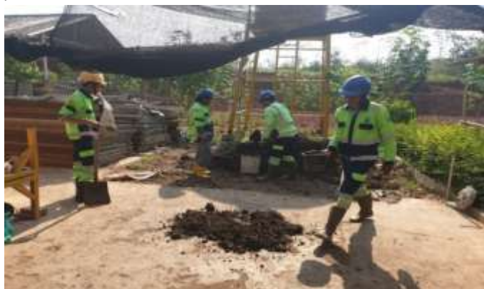
Figure 2. Compost Block Production Process from Locally Available Biomass and Organic Materials
