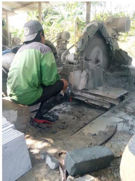
Picture 2. Process cutting rock natural use machine grinder cut in location production Dhafin Stone (Source: Dhafin Stone Documentation, 2026)
