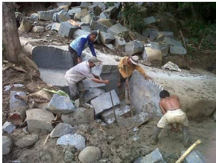
Picture 1. Process mining And cutting beginning chunks rock natural in a way manual (Source: Dhafin Stone Documentation, 2026)
