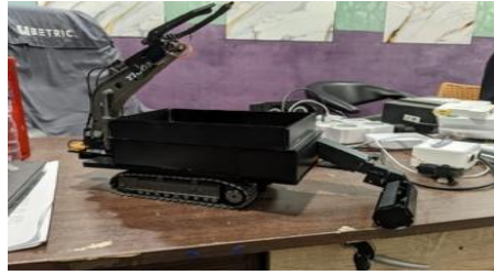
Figure 8. Prototype of the Oil Palm Fruit Collection Robotic Automation System
